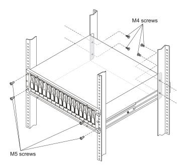
Figure 20. Securing the DS5020 to the rack cabinet
